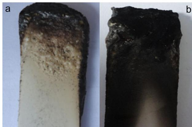
**Figure 7.** The char morphology of the burned bars (UL94 test, the flame time: 20 s) of (a) MPP/GFRPA6 and (b) MPP/SPR/GFRPA6.
